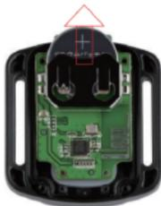
Note: Do NOT rotate the PCB board to avoid reversing the camera and video button functions.
